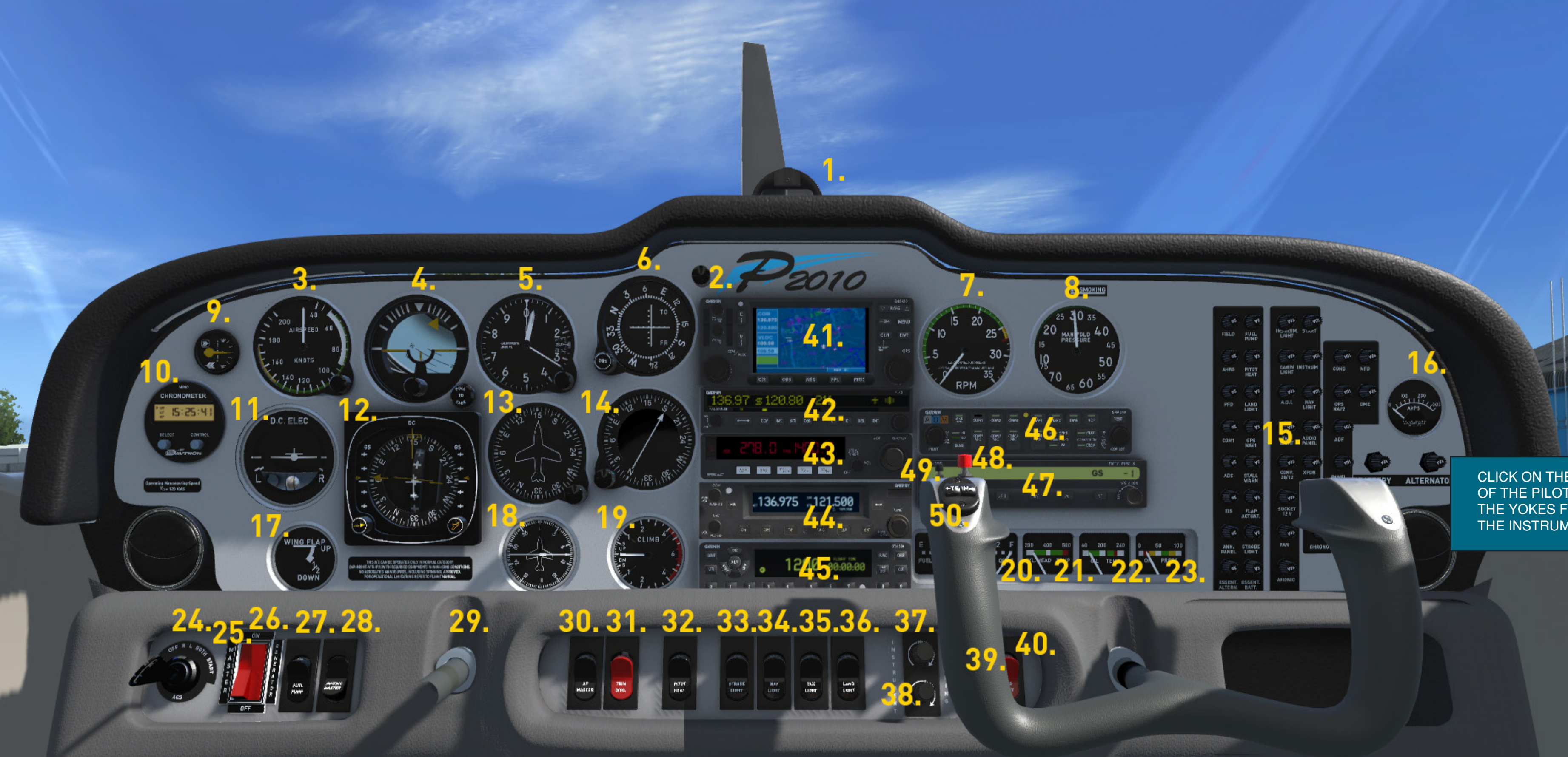
1. Compass 2. NAV/GPS Switch 3. Airspeed Indicator 4. Artificial Horizon 5. Altimeter (VSI) 6. OBS 7. Tachometer 8. Manifold Pressure 9. Trim Indicator 10. Chronometer 11. Turn/Slip 12. HSI 13. Gyro Compass 14. RMI (NAV1) 15. Circuit Breakers 16. Generator Amps 17. Flap position Indicator 18. Radio Compass (ADF) 19. Climb/Fall Indicator (VSI) 20. Fuel Contents 21. Cylinder Head Temp. 22. Oil Temp. 23. Oil Pressure 24. Magneto/Starter 25. Master Battery 26. Generator 27. Fuel Pump 28. Avionics Master 29. Toggle Yoke Vis. 30. AutoPilot Master Switch 31. Secure Aircraft (Chocks etc.) 32. Pitot Heat 33. Strobe Lights 34. Nav. Lights 35. Taxi Light 36. Landing Light 37. Instrument Light Dimmer 38. Panel Lights 39. (hidden) Pilot Removal 40. Cabin Lights
