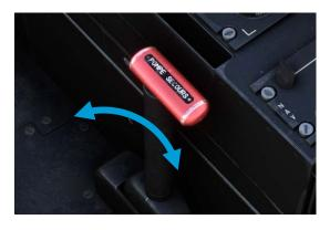
4. Stop pumping once the three landing gear lights are green.
