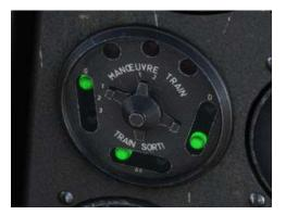
It is not possible to retract the landing gear using emergency circuit.
