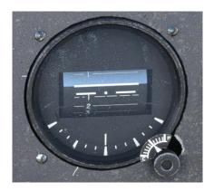
This instrument will indicate pitch angle between 0 and 80 degrees and bank angle with a graduation each 10 degrees between 0 and 60 degrees.
