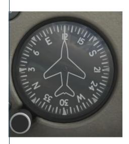
The heading indicator is your primary reference for flying particular headings. Over time, the heading indicator will drift out of proper alignment. Your instructor will help you check that your instrumentation remains aligned with the magnetic compass and point out if significant drift is present.
