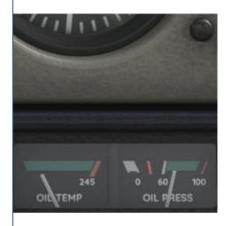
Normal operation of the engine oil system is indicated by the temperature and pressure gauges displaying their needles in the green band. High oil temperature or low oil pressure indicate an issue with the engine, so this must be monitored periodically to ensure that any unusual indications are spotted quickly, allowing time to troubleshoot and perform a precautionary landing if necessary.
