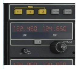
The C152 is fitted with two communications (COMM) radios. Each radio is fitted with an active/use window and a standby window. Turning the inner and outer knobs to the bottom right of the radio allows for tuning of the standby frequency. Once correctly set to the desired frequency, pushing the white swap button (<->) swaps the standby frequency with the active frequency. We will be primarily using the COMM1 radio, which is located at the top left of our radio stack.
