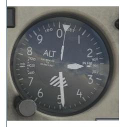
Normally set to display altitude Above Mean Sea Level (AMSL) the altimeter displays your vertical height in feet. Maintaining accurate altitude control is especially important when flying through or near to airspace boundaries, as we often avoid entering controlled airspace by flying at an altitude below the floor of airspace above us.
