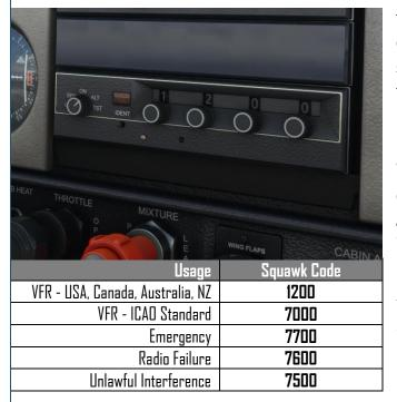
The transponder (often shortened to XPDR) of our Cessna 152 can be found at the base of the radio stack and is set to a 'squawk' code of 1200. This is the standard code in the USA and some other locations to label us on the ATC radar screen as a light aircraft flying under Visual Flight Rules (VFR) and is referred to as the 'conspicuity' code.
