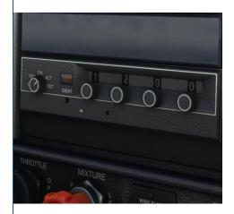
The code we set into the transponder is known as our 'squawk' code and is visible on the Air Traffic Control (ATC) radar screen. To set the squawk, turn the knobs located under each number, which have a range of 0-7. Lighting conditions in Flight Simulator can often make the transponder difficult to read, so you may need to zoom in to get a clear view. Leave the transponder mode knob in the Altitude Reporting (ALT) position.
