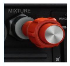
Beside the throttle you will find the mixture control. When flying at higher altitudes the air becomes thinner. As the engine runs most efficiently at a certain fuel:air ratio, we reduce the fuel flow slightly after climbing in order to preserve this ideal ratio. This ensures proper engine running and fuel efficiency.
