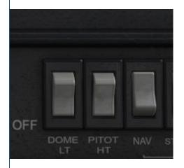
As discussed above, you may need to hide the yoke in order to get a clear view of the pitot heat switch, which is located at the bottom of the instrument panel, towards your knees. To the left of the pitot heat switch is the dome light switch, which can be turned on if you find cockpit lighting conditions to be too dark, depending on your display and graphics settings.
