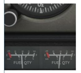
Located beneath the heading indicator there are a pair of fuel gauges which display the remaining fuel quantities for both the left and right fuel tanks, located in the wings.
