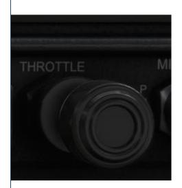
Speed control is achieved by use of the throttle lever. Make smooth adjustments to the throttle in order to change speed, as rapid movements make sudden changes to speed and lift, which can make altitude holding more challenging.
