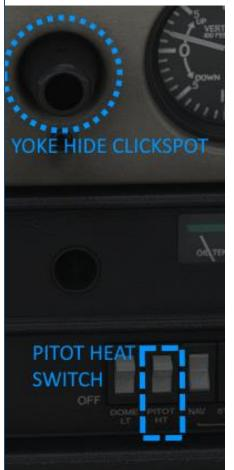
Inflight protection is also required, as icing can block the air intakes of critical instrumentation, rendering them useless. To protect our airspeed indicator, we have the pitot heating system, which electrically heats the pitot tube, used to measure the pressure of the oncoming airflow for conversion to an indicated airspeed. If our pitot tube becomes blocked with ice, the pitot tube will no longer be able to detect oncoming airflow and so our airspeed indication will drop to zero.
