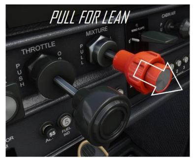
The engine is considered to be running 'rich' if too much fuel is being supplied. This can cause carbon deposits within the engine and cause rough running and poor fuel economy.
