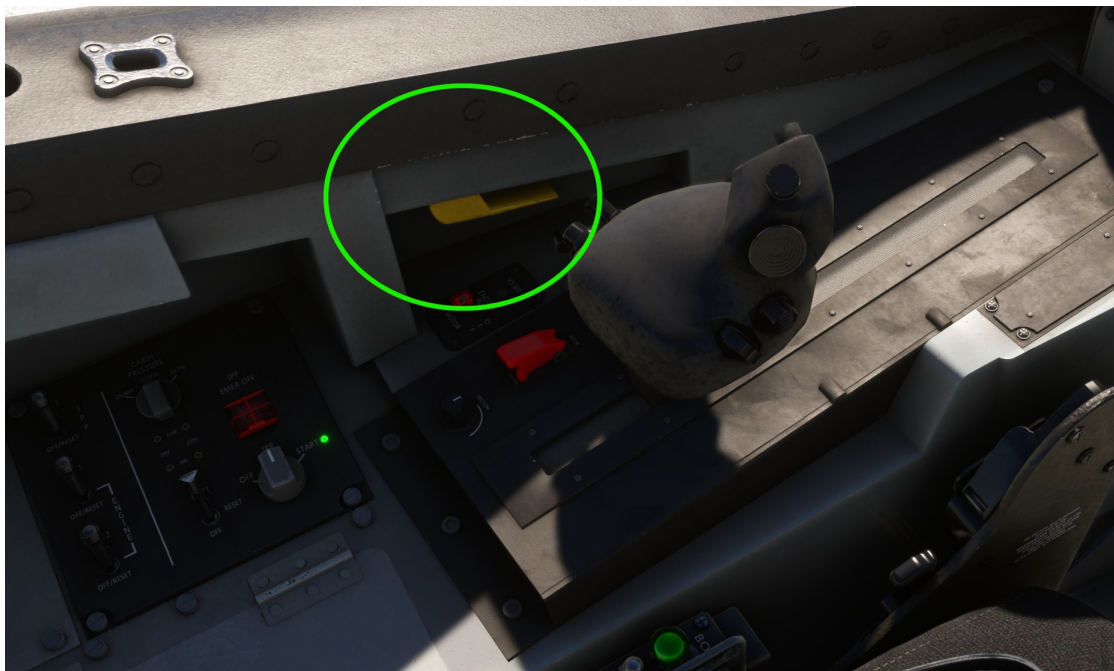
Location of canopy control lever – NOTE: in the real aircraft this is the canopy LOCK lever: a separate "UP-DOWN" switch is located nearby.
