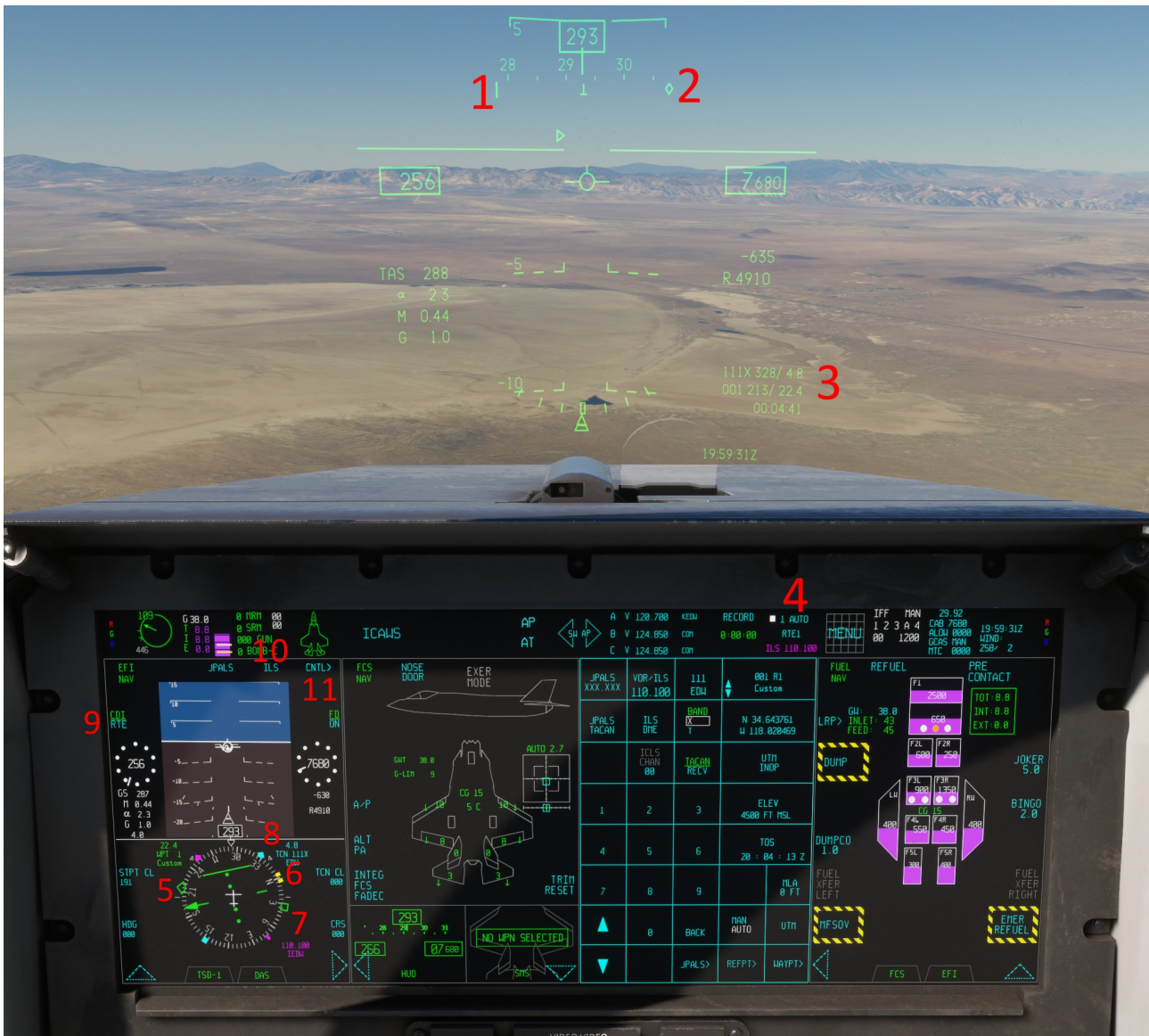
The picture above shows a situation in which the selected NAV source is RTE, and the aircraft is also receiving signals from the VOR and TACAN receivers.
