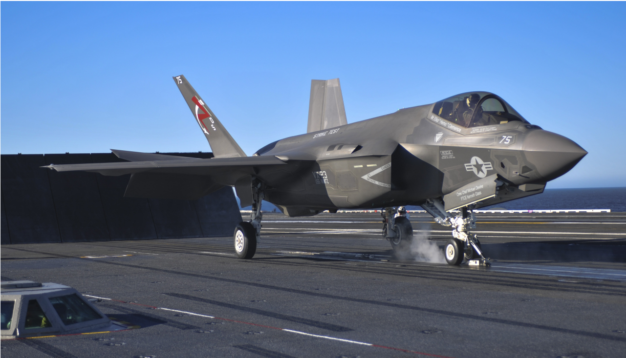
F-35C in preparing for a catapult-assisted take-off from a USS Nimitz-class carrier
