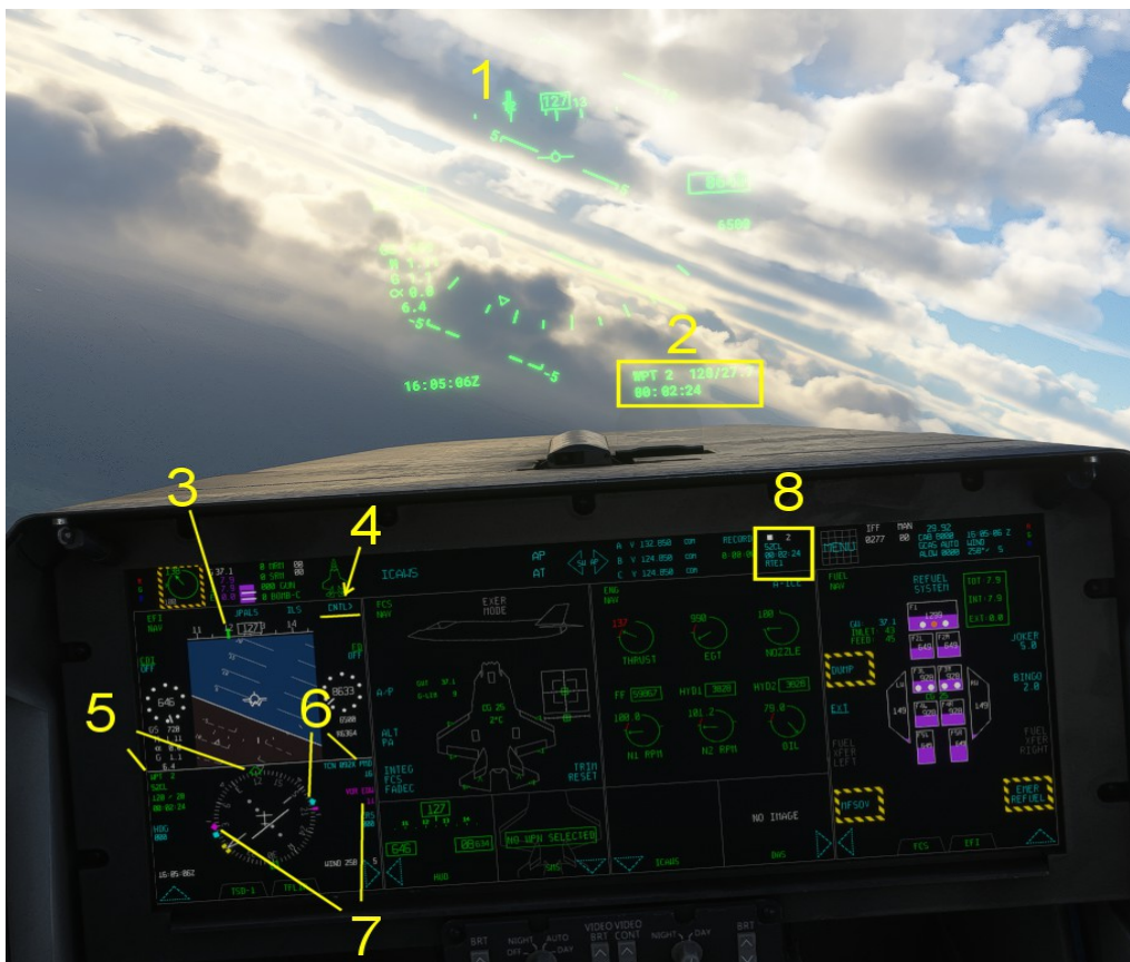
The picture above shows a situation in which the selected NAV source is RTE, and the aircraft is also receiving signals from the VOR and TACAN receivers.
