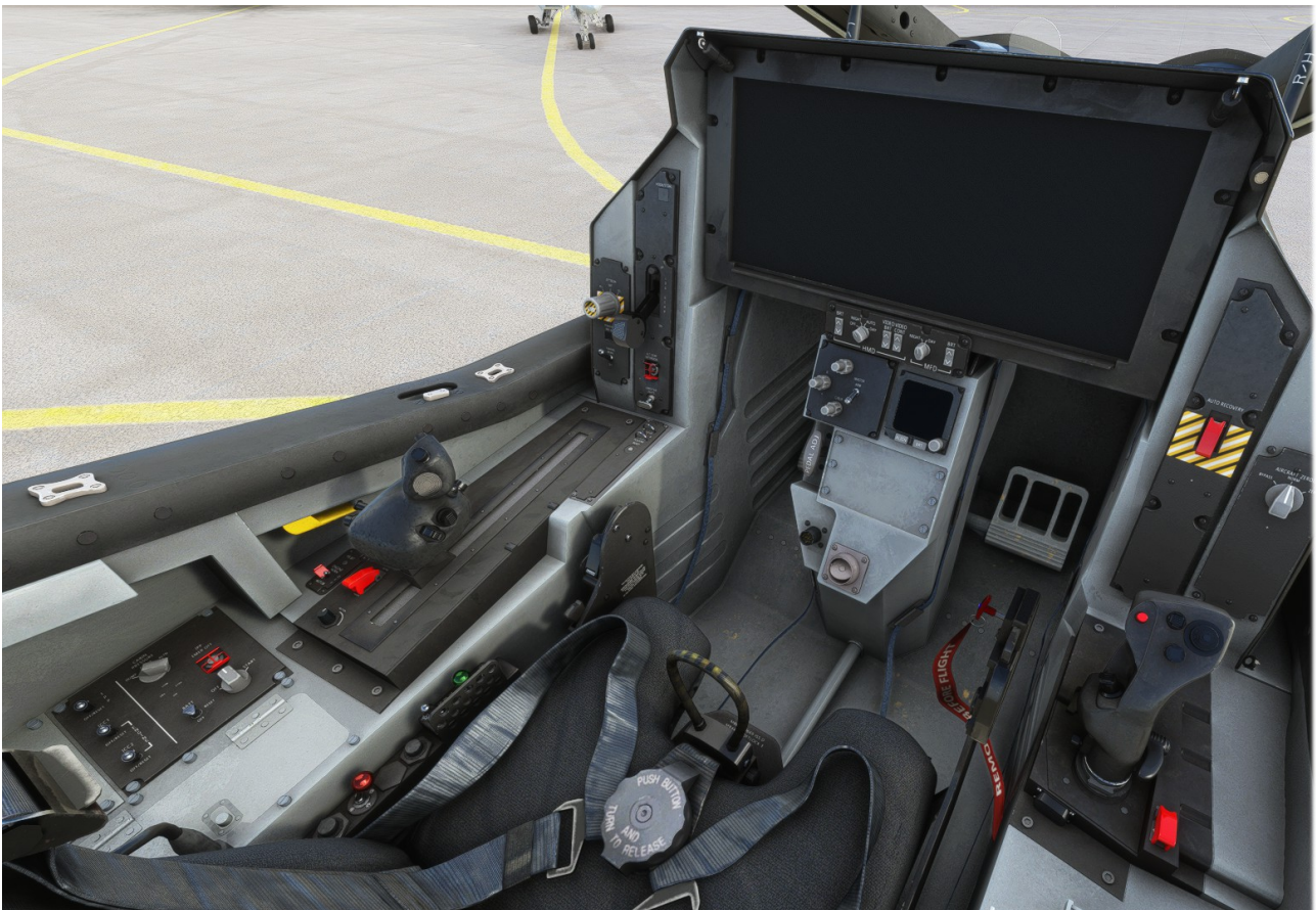
COCKPIT GENERAL VIEW – cockpit layout is identical for -A, -B and -C variants. The geometry of -B variant cockpit is slightly different, with poorer backward visibility, to make room for the Lift-Fan system intake.
