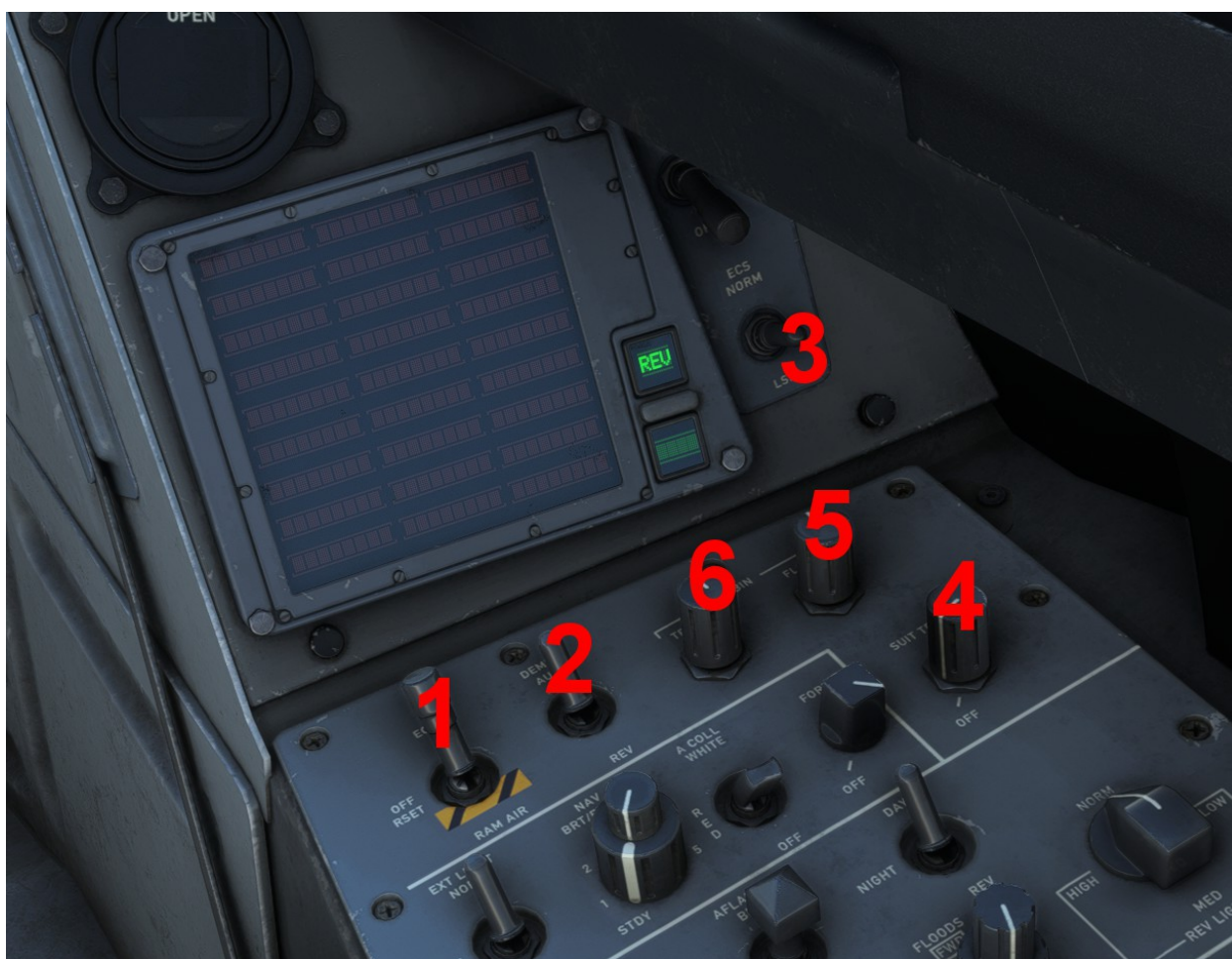
Environmental Control System Controls
