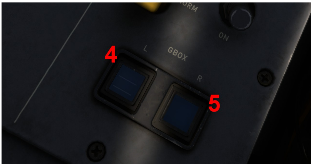
4 Left Gearbox Air Drive Push-button; 5 Right Gearbox Air Drive Push-button
