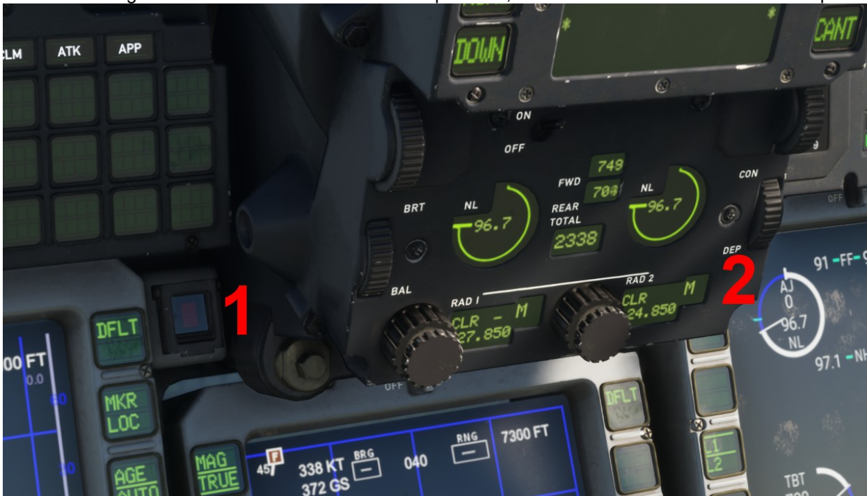
FIRE INDICATORS / PUSHBUTTONS
