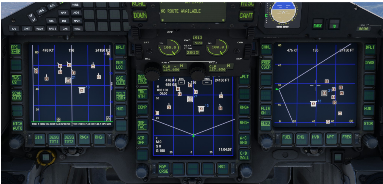
TYPICAL AIR-TO-AIR MHDD CONFIGURATION
