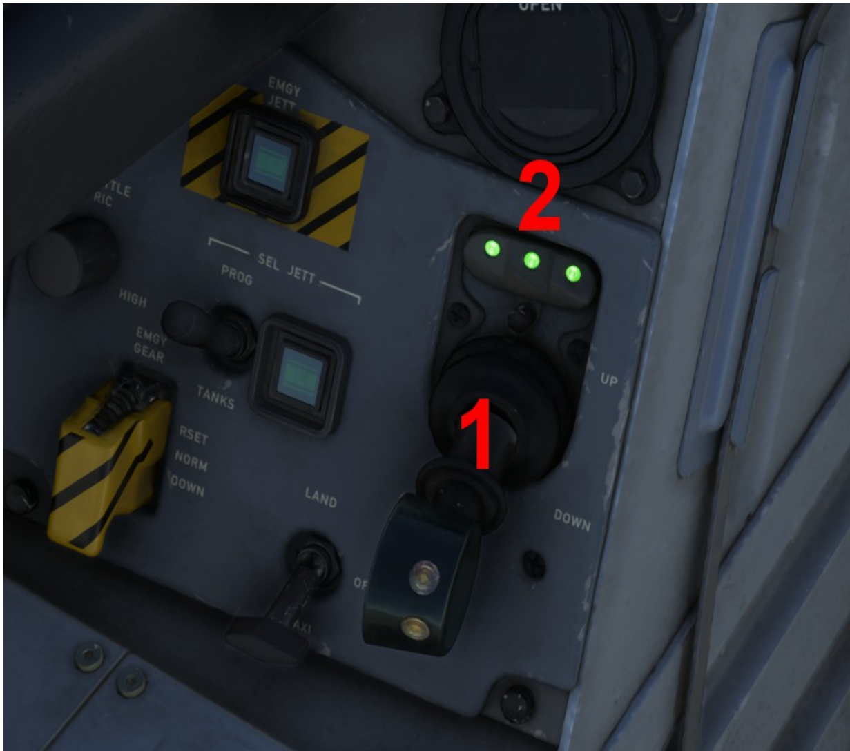
LANDING GEAR CONTROLS (Left quarter panel)
