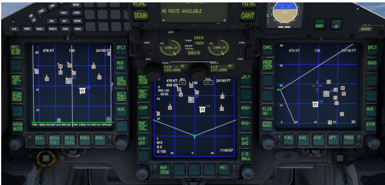
TYPICAL AIR-TO-AIR MHDD CONFIGURATION
