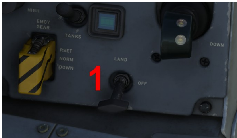
1 – LANDING/TAXI LIGHT (Left quarter panel)
