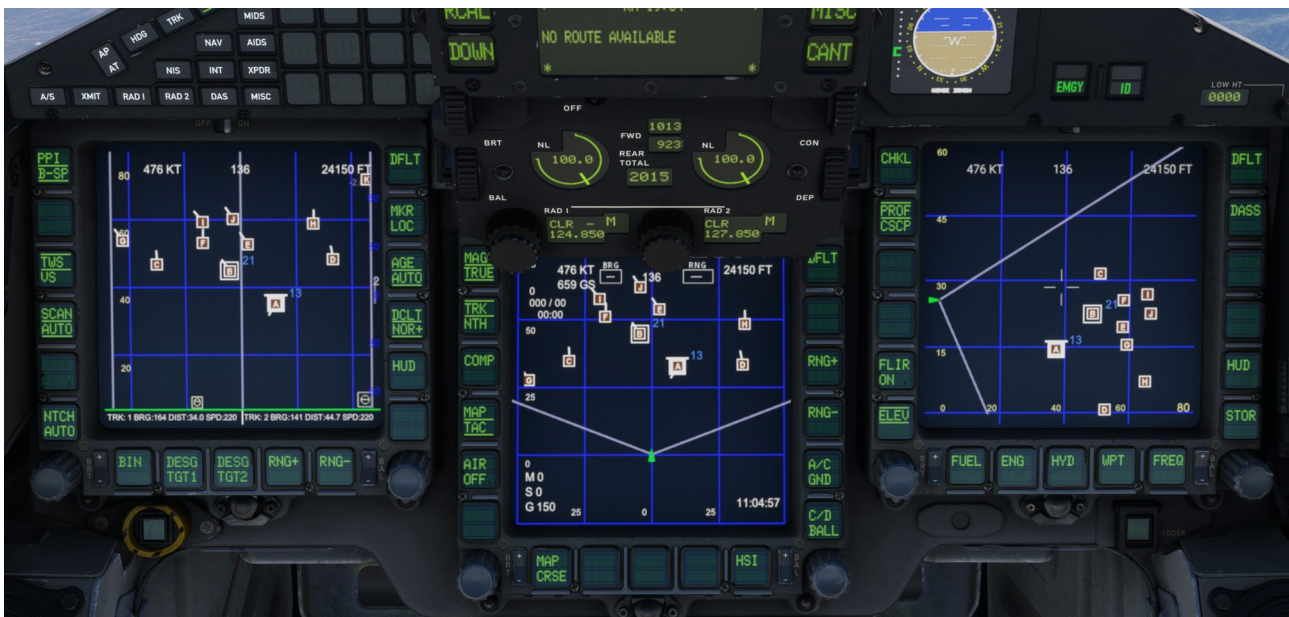
TYPICAL AIR-TO-AIR MHDD CONFIGURATION
