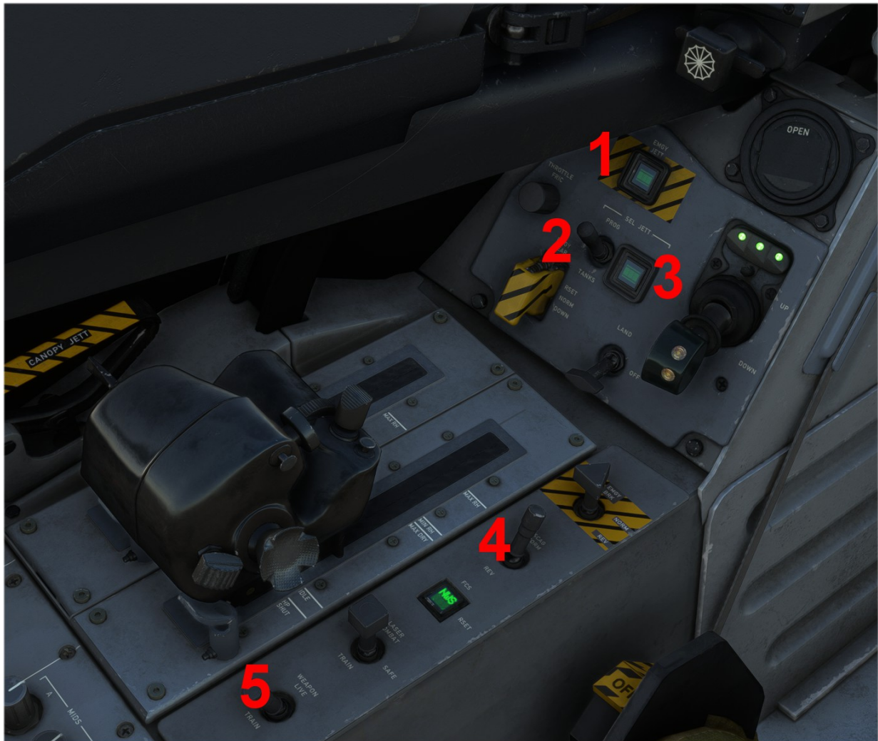
ACS controls/indicator (left consoles)
