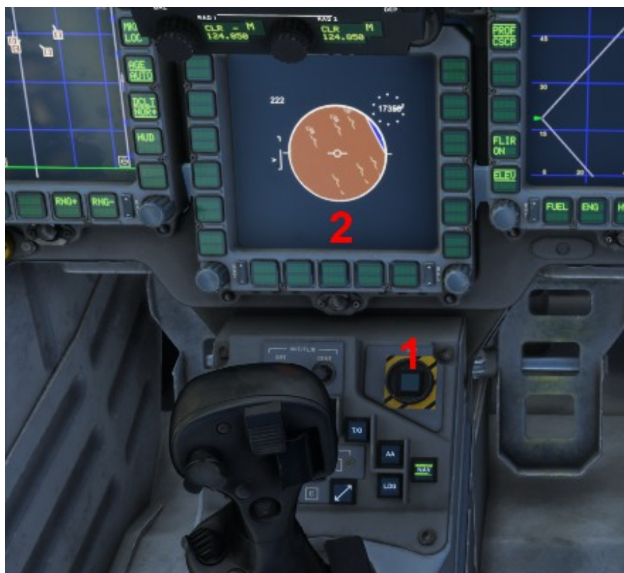
DISORIENTATION RECOVERY CONTROLS AND DISPLAYS
