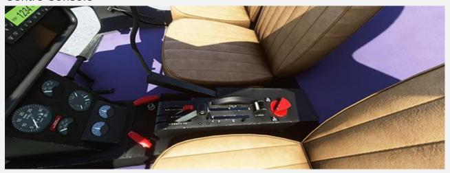
The center panel houses the Throttle and Mixture levers which control the engine power to the aircraft.
