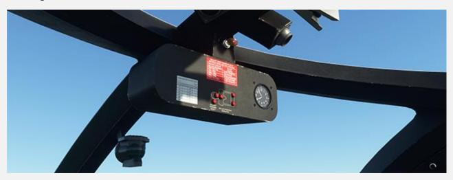
This houses the ballast warning system, reference cards, clock and whisky magnetic compass.
