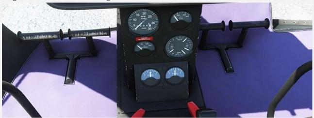
In the front center console are the engine and fuel gauges.
