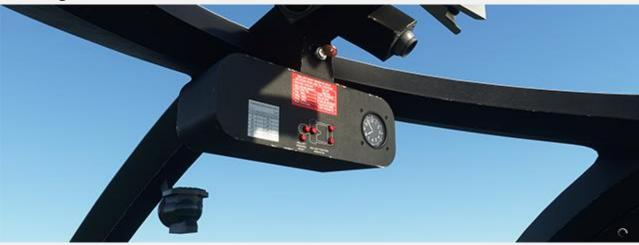
This panel has the reference card for the ballast weight system, below that is the warning panel if the ballast in incorrectly placed and centre of gravity it out of balance, a clock and the magnetic deviance reference card.
