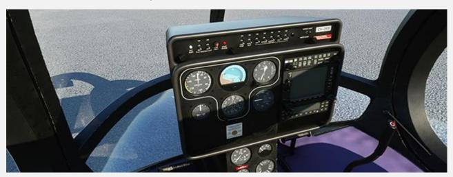
This houses the standard aircraft switches for electrics and lighting, primary flight instruments, audio selection unit, the Garmin GNS 530 GPS navigation unit and the Garmin GTX330 transponder unit.
