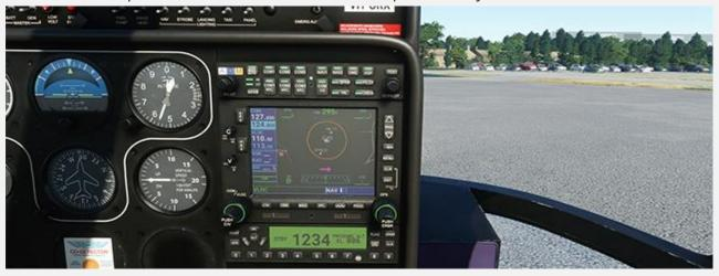
To the right of the 6 pack are the audio and navigation panels allowing for comms to be switched, volumes adjusted and functions selected.
