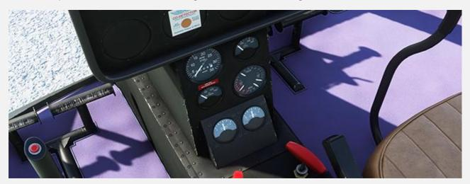
In the middle of the seats in the centre panel are the main fuel cut-off levers, throttle and mixture levers, trim wheel, flaps switch, wheel brakes and fuel selection switch.
