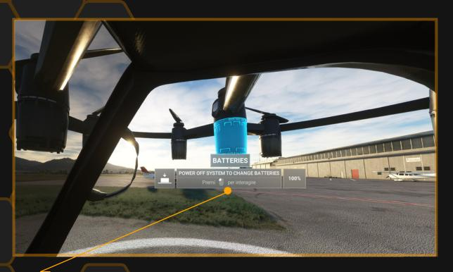
With power off, click right (or left) battery cover to change batteries.
