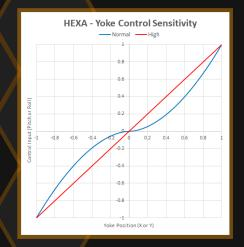
The graph on the left shows how the two different sensitivity modes affect the yoke sensitivity.
