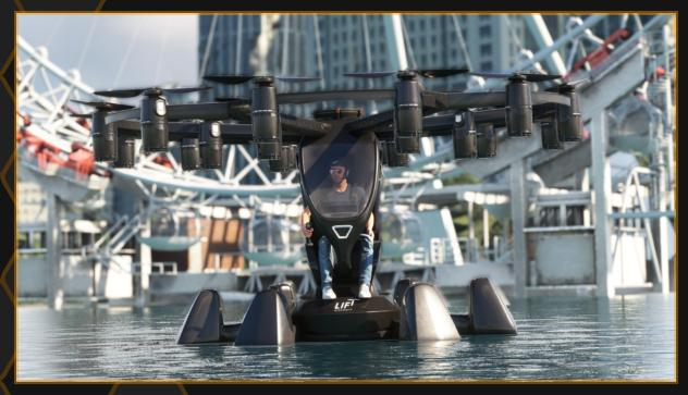
HEXA is a full Fly-By-Wire electric Vertical Takeoff and Landing (eVTOL) aircraft designed to be piloted by anyone and experience the thrill of vertical flight!
