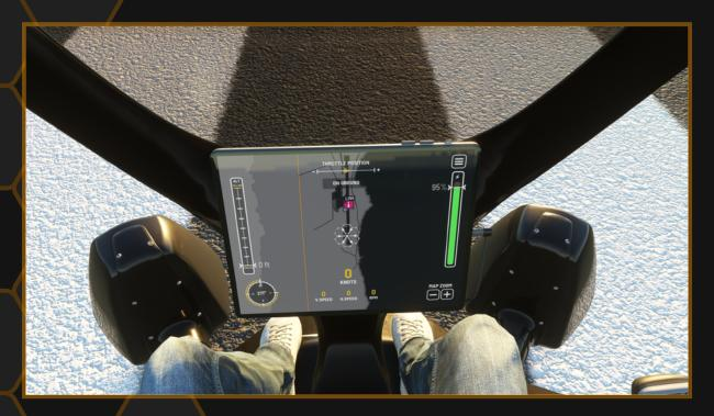
Being the aircraft full FBW, the throttle slider works as an indirect rpm variation control.
