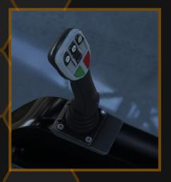
Hexa's yoke allows you to control the drone pitch and roll, and gives you access to some very interesting functions: auto take-off and auto-landing. Once you have pressed the corresponding button on the top of the yoke, if the conditions for initiating those procedures are met a message will appear on the tablet, asking you to confirm or abort the requested procedure via the green on red buttons on the yoke, or tapping on the corresponding icons on the tablet screen.
