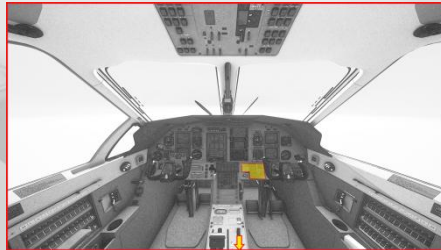
Cabin Pressurisation Control System (CPCS)
